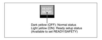
Normally, this button is dark yellow (READY SETUP is off). In this case, the buttons, controls and switches directly control the audio processing.
